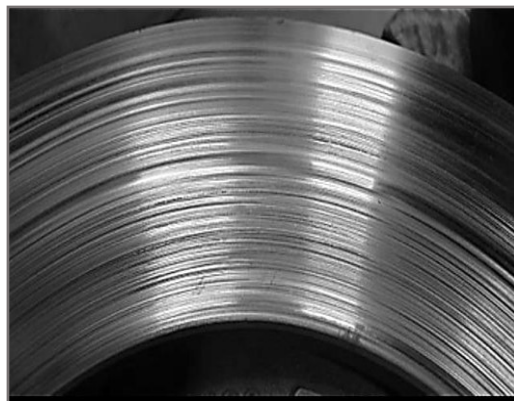
FIGURE 7. Grooves on Brake Surface
